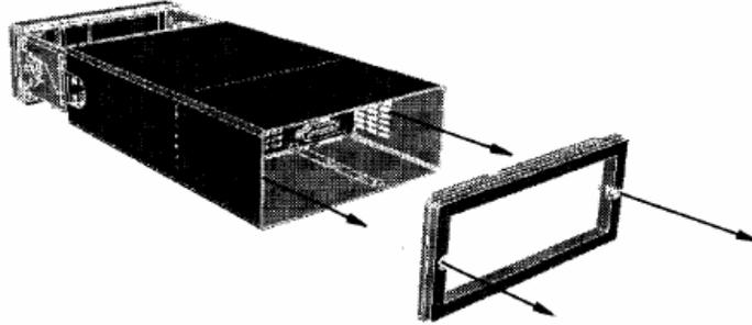
To remove the cover, remove the two screws that hold the rear bezel, as shown in the above picture.
