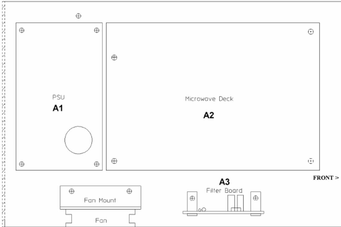
Figure 6-3 Layout of A2 Block Down Converter
