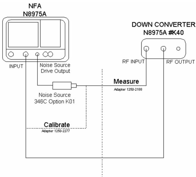
**Figure 4-2** Test Set-up for LO Accuracy and Troubleshooting
